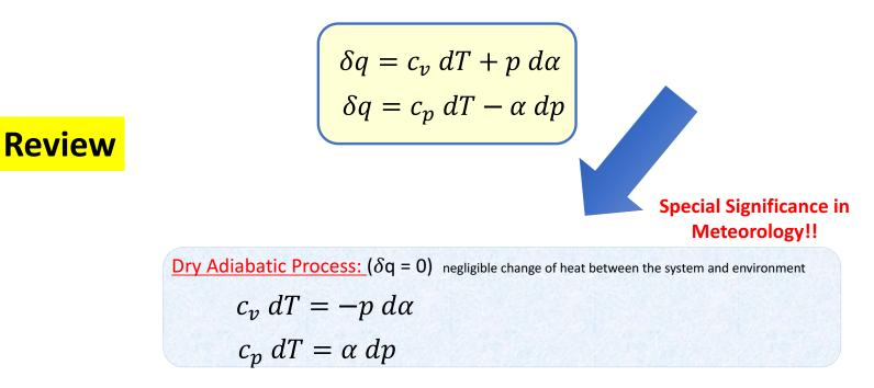
No condensation or evaporation occurs and no heat is added to or removed from the parcel of air, as the parcel moves up and down in atmosphere!
