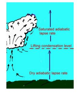
Key fact: When a parcel moves through the atmosphere dry adiabatically, its temperature follows a dry adiabat and the dewpoint follows a saturation mixing ratio line. The lifting condensation level (LCL) of the parcel is defined by the pressure level where these two lines intersect. If the parcel reaches the LCL adiabatically, it will become saturated. If it continues to rise adiabatically, its temperature and dewpoint will be the same, both following a moist adiabat.
