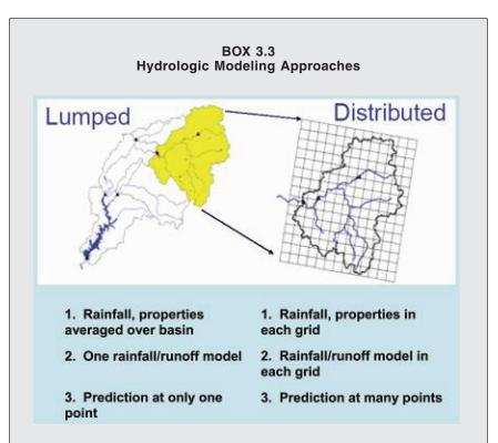
FIGURE Comparison of lumped and distributed hydrologic modeling approaches. SOURCE: NRC (2006b).
