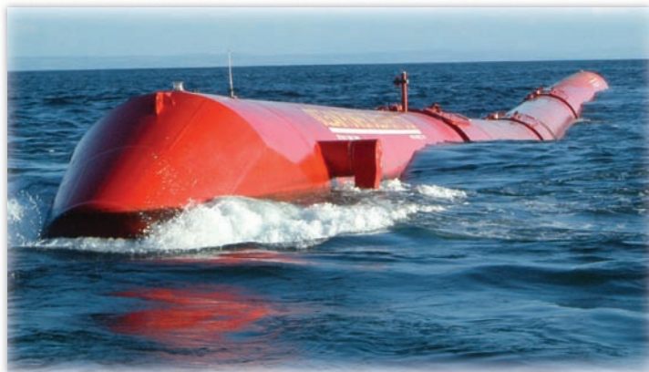
▲ FIGURE 13.34 The Pelamis wave converter (named after a sea snake) is a 125 m long and 3.5 m diameter tube, hinged so it undulates as ocean swells pass along it. This motion drives pistons that turn electrical generators. Energy experts calculate that capturing just 1 to 2 percent of global wave power could supply at least 16 percent of the world's electrical demand.
