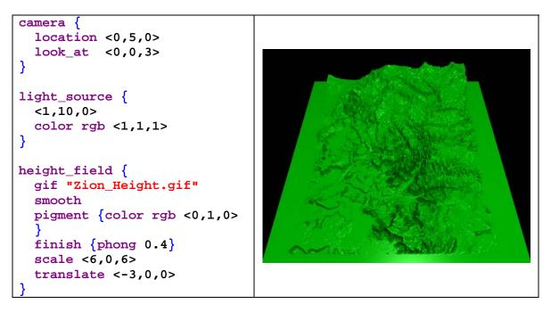
An important note to make is that with POV-Ray we are not limited in where we can place our camera location whereas in GMT our camera location is constrained to be off at infinity. So, for example, we can zoom in to very unique views.
