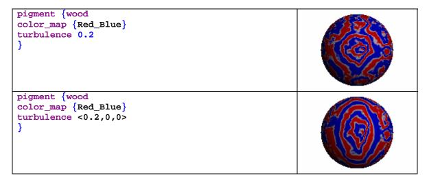
Here we applied the **turbulence** command to our wood example from above. The first example applied equal amounts of turbulence (defined in the range from 0.0 to 1.0) in all directions. The second example only applied turbulence in the x-direction.
