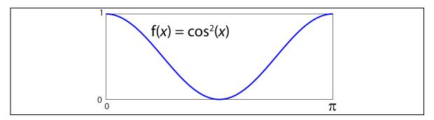
Let's just consider the interval from 0 to  $\pi$ . We can determine the value of this integral analytically as  $E = \pi/2 \sim 1.5708$ .
