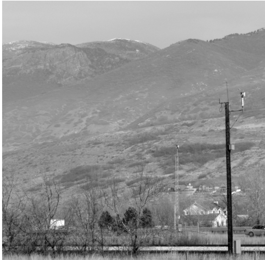
Figure 2: Anemometers installed in Centerville, UT, by Union Pacific Railroad (MesoWest identifier: UP028; foreground) and Utah Department of Transportation (MesoWest identifier: CEN; background), at the location of strongest observed winds during the 1 December 2011 windstorm.
