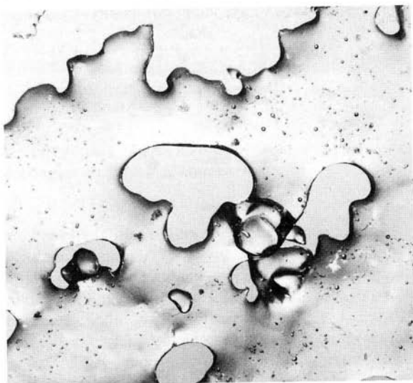
Figure 3.19. Thin sections of snow illustrating newly fallen snow, old dense snow (rounded forms), and a thin ice crust. (Photos by E. LaChapelle)
