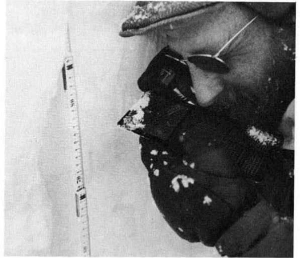
Figure 3.7. Definition of snow layers with shovel, brush, and edge of crystal screen. Use of a hand lens and millimeter crystal grid for examining snow crystals (bottom right). Magnification of 8 to 10X is recommended for field use.
