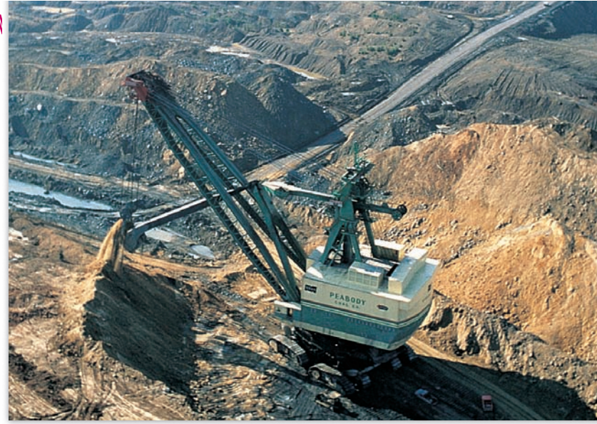
▲ FIGURE 12.13 Some giant mining machines stand as tall as a 20-story building and can scoop up thousands of cubic meters of rock per hour.
