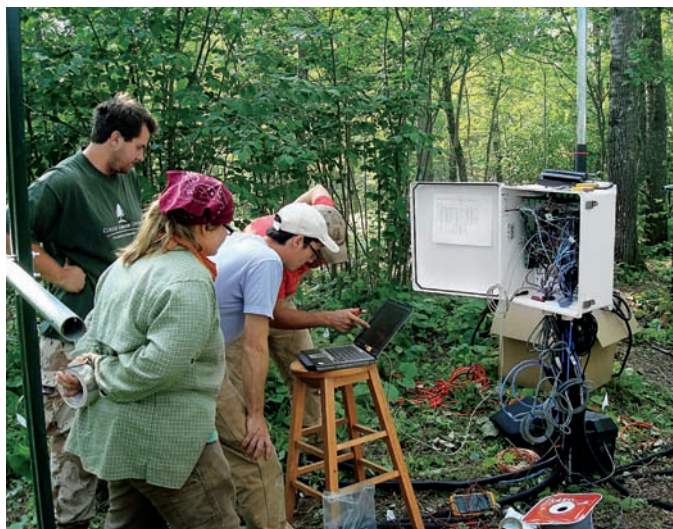
◀ FIGURE 5.2 Students and technicians adjust the electrical panel that controls heat lamps and heating cables. SOURCE: Peter Reich.
