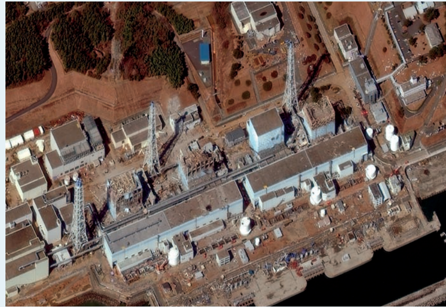
▲ Three of the four nuclear reactors at Japan's Fukushima Daiichi that were destroyed by fuel melting and hydrogen explosions after the 2011 tsunami knocked out emergency cooling systems.
