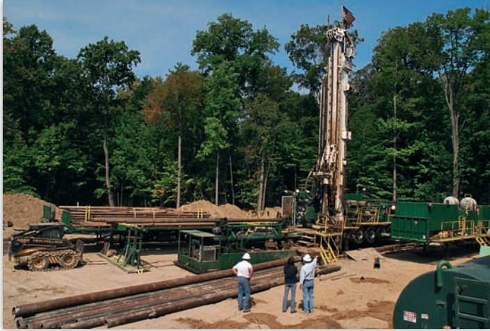
▲ FIGURE 12.12 Hundreds of thousands of natural gas wells have been (or are being) drilled in the United States. Often, these wells require a controversial procedure called hydraulic fracturing, or fracking, to release gas from sedimentary formations.
