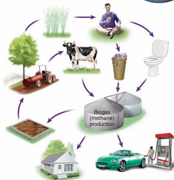
▲ FIGURE 14.1 Biogas plants convert all types of organic waste into usable methane and fertilizer.
