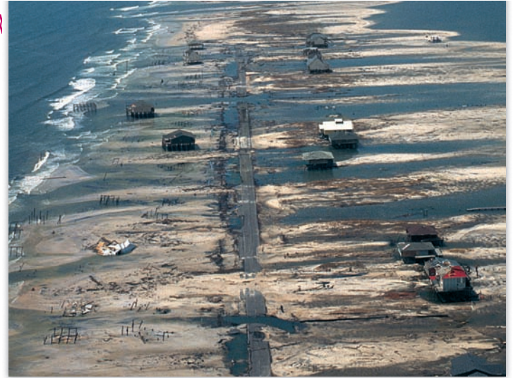
▲ FIGURE 12.22 The aftermath of Hurricane Katrina on Dauphin Island, Alabama. Since 1970, this barrier island at the mouth of Mobile Bay has been overwashed at least five times by storms. More than 20 million yd 3 (15 million m 3 ) of sand have been dredged or trucked in to restore the island. Some beach houses have been rebuilt, mostly at public expense, five times. Does it make sense to keep rebuilding in such an exposed place?
