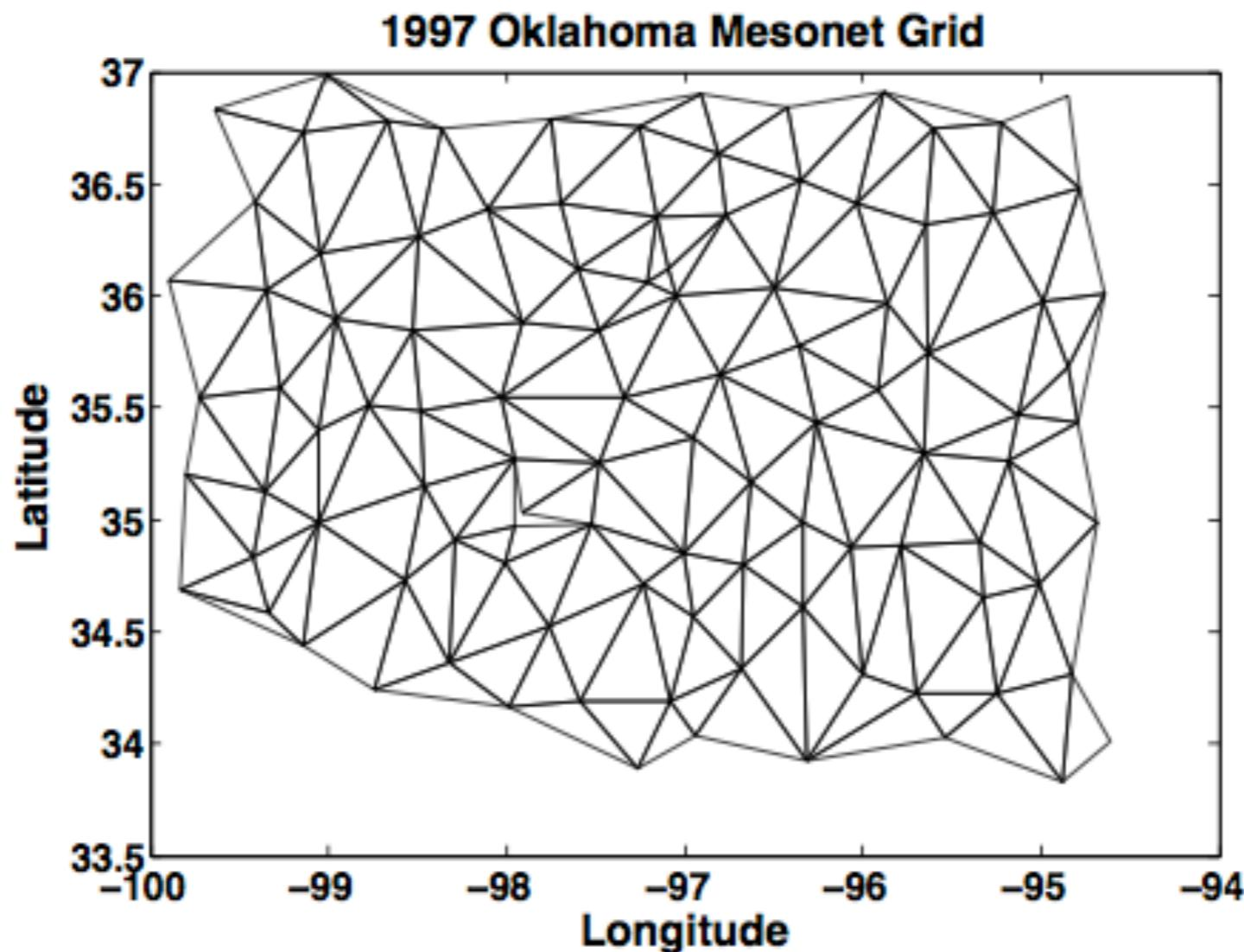
Fig. I. Map of the Oklahoma Mesonet grid used for 1997. Delaunay triangulation was used to connect the stations to form the grid. Low aspect ratio triangles were removed, primarily on the outer border with the exception of two near 35°N 98°W.
