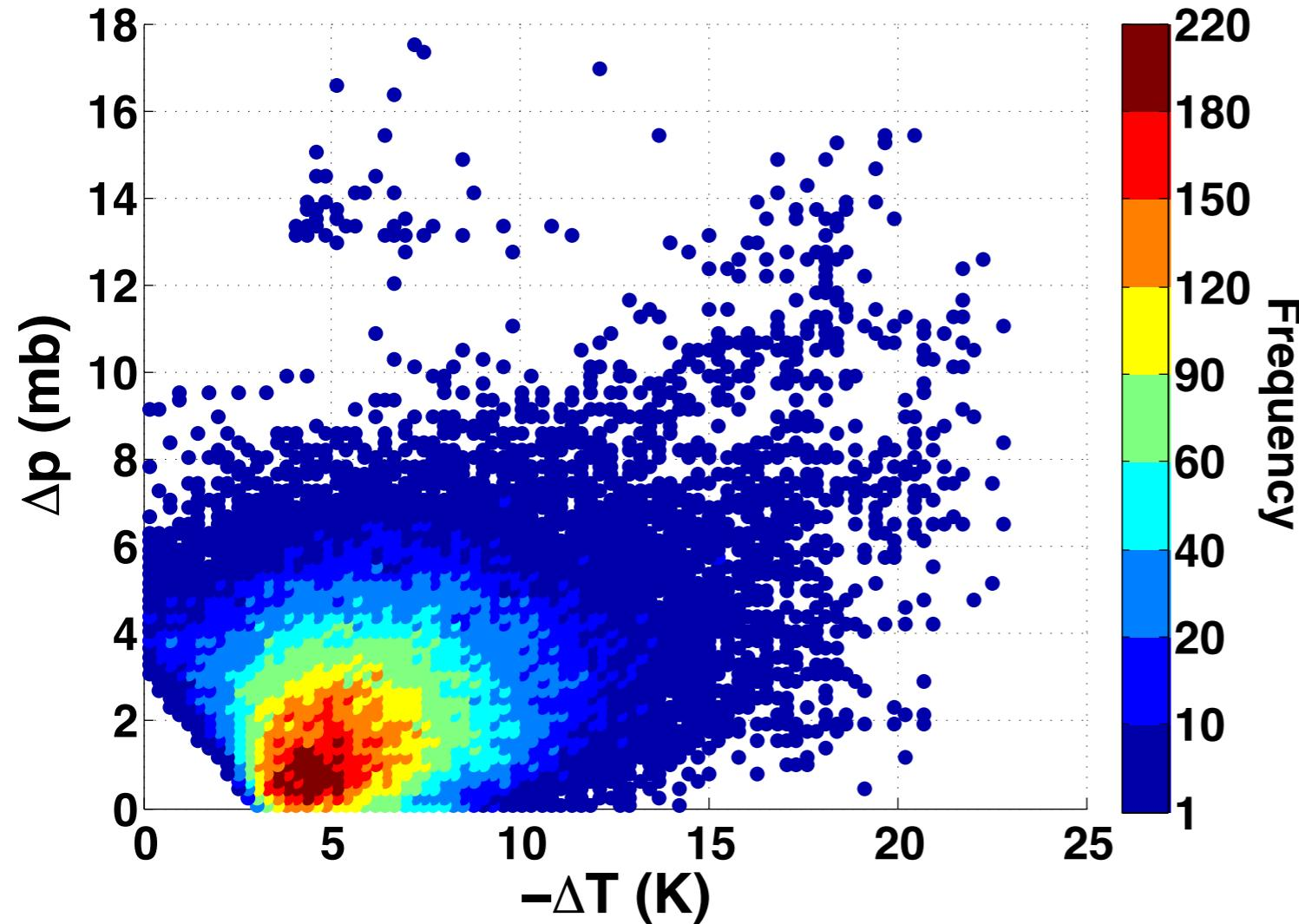
Fig. 14.  $\Delta p$  versus  $-\Delta T$  at stations that are part of frontal passages across triangles in the Oklahoma Mesonet from the 1997-2011 period. The color bar represents the frequency of occurrence. The correlation is 0.28.
