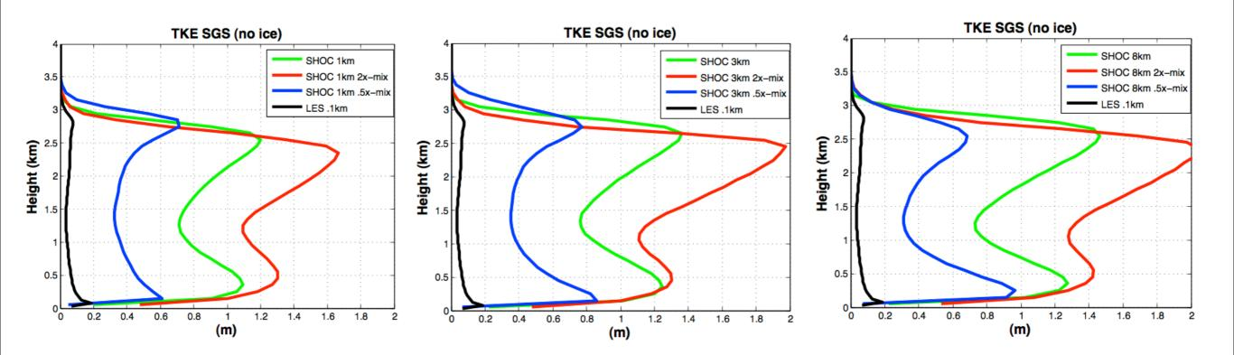
All three have a similar result with a lower mixing ratio bringing SGS TKE closer to the LES.
