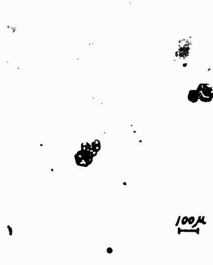
b. Ice crystals nucleated at -22^{\circ}\text{C} from the supercooled droplets, 100 m from the power plant stack.
