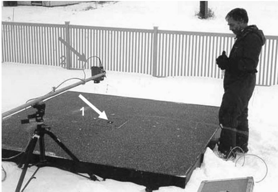
Fig. 1. The experimental set-up consisted of a 2.4 m \times 2.4 m black plywood base with a detector mounted in the center (arrow 1) that measured transmitted irradiance. Incident and reflected irradiance were measured using a second detector that was mounted on a tripod (arrow 2).
