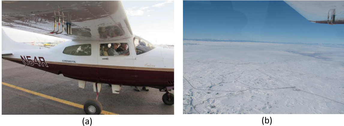
Figure 4-1. Photographs of the Cessna 210 aircraft that sampled over the Uinta Basin in February 2013. (a) Three inlets and two temperature and humidity probes were installed under the starboard wing. (b) View of the snow covered Uinta Basin from the aircraft.
