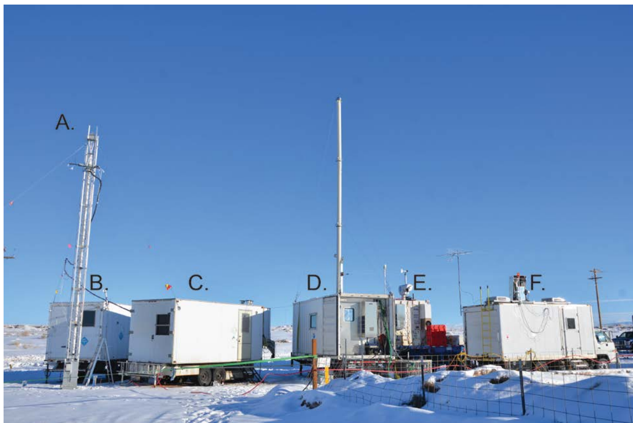
5-1. A picture of the UBOS 2013 Horse Pool Intensive site facing North. The individual components are (A) sample tower with automated inlet, (B) NOAA/CSD nitrogen species trailer, (C) NOAA/CSD VOC trailer, (D) NOAA/PMEL aerosol and snow lab, (E) NOAA/CSD HRDLS trailer, (F) NOAA/CSD TOPAZ trailer. Photo credit, Scott Sandberg.
