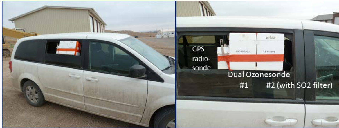
Figure 8-31. Ozonesondes mounted in the window of a NOAA van used to measure ozone concentrations while driving around the Uinta Basin. This photo was taken during the 2012 study but a similar configuration was used in 2013.
