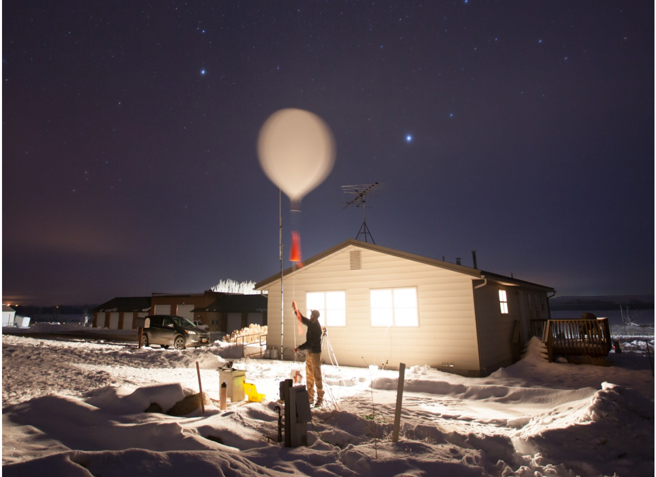
Figure 8-3. A portable NOAA automated ozonesonde tether installation in operation in the late evening at the Ouray Wildlife Refuge site. This system was operated remotely from within the staff house that also served as an ozonesonde preparation and calibration center. Photo: Patrick Cullis, NOAA/CIRES, February 2013.
