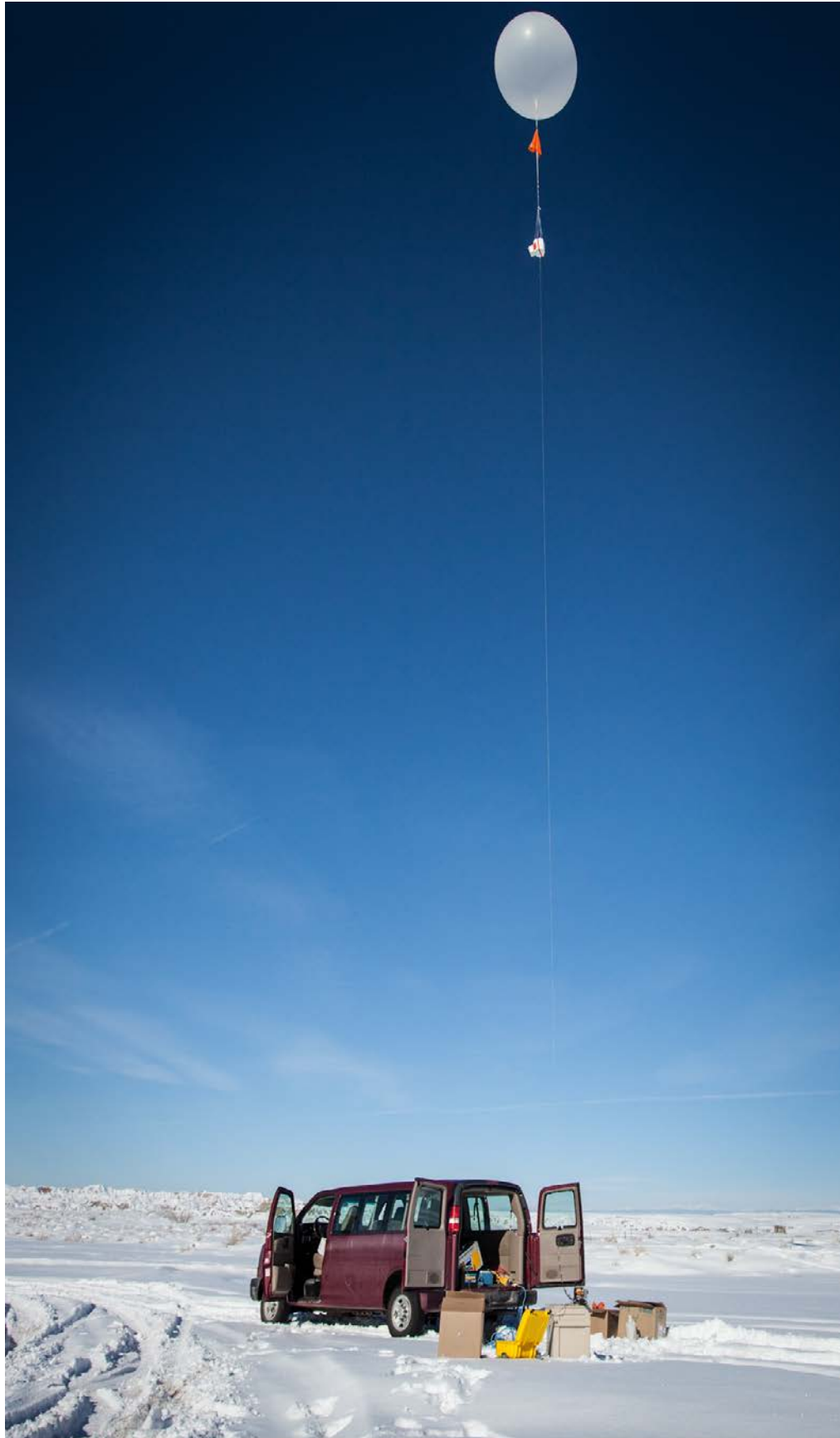
Figure 8-2. An automated, portable NOAA tethered ozonesonde system at the Fantasy Canyon site. The tethered ozonesonde system was set up and in operation within an hour of arriving on site. The complete system is battery operated and can be left alone to conduct profiles to a pre-set altitudes, then return to the surface before repeating the cycle. The system will run for ~4 hours before sonde batteries require changing. Photo: Patrick Cullis, NOAA/CIRES, February 2013.
