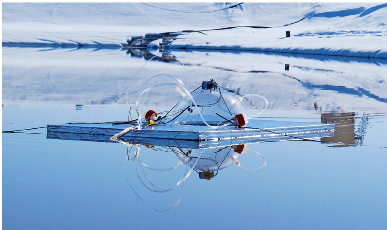
Figure 9-6. USU dynamic flux chamber on a produced water pond.
