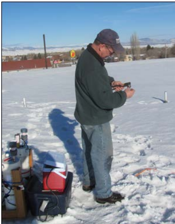
Figure 3-2. Hand-held methane (CH 4 ) vial collection and paired VOC sorption tube collection (red ice chest) at the Vernal, Highway 40 sampling location.
