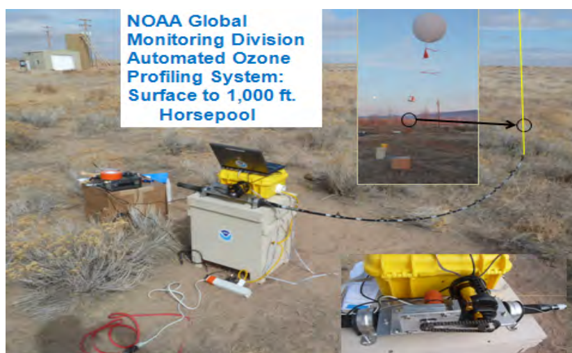
Figure 5B-1a. The portable automated ozonesonde tether setup at Horse Pool.
