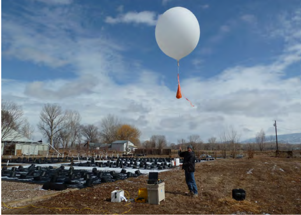
Figure 5B-1b. The portable automated ozonesonde tether setup at Jensen, Utah.
