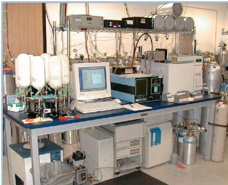
Figure 5A-5. NOAA MAGICC flask analysis system. Every year, the MAGICC lab analyses over 20,000 air samples collected by scientists and volunteers at a global network of surface sites and a North American network of tall towers, aircraft vertical profile and intensive study sites ( http://www.esrl.noaa.gov/gmd/dv/iadv/ ).
