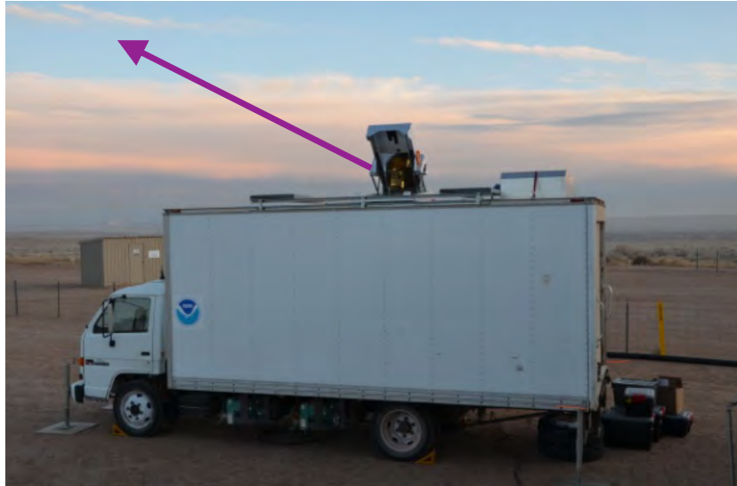
Figure 3-49. Truck-mounted TOPAZ ozone lidar with roof-top, two-axis scanner.
