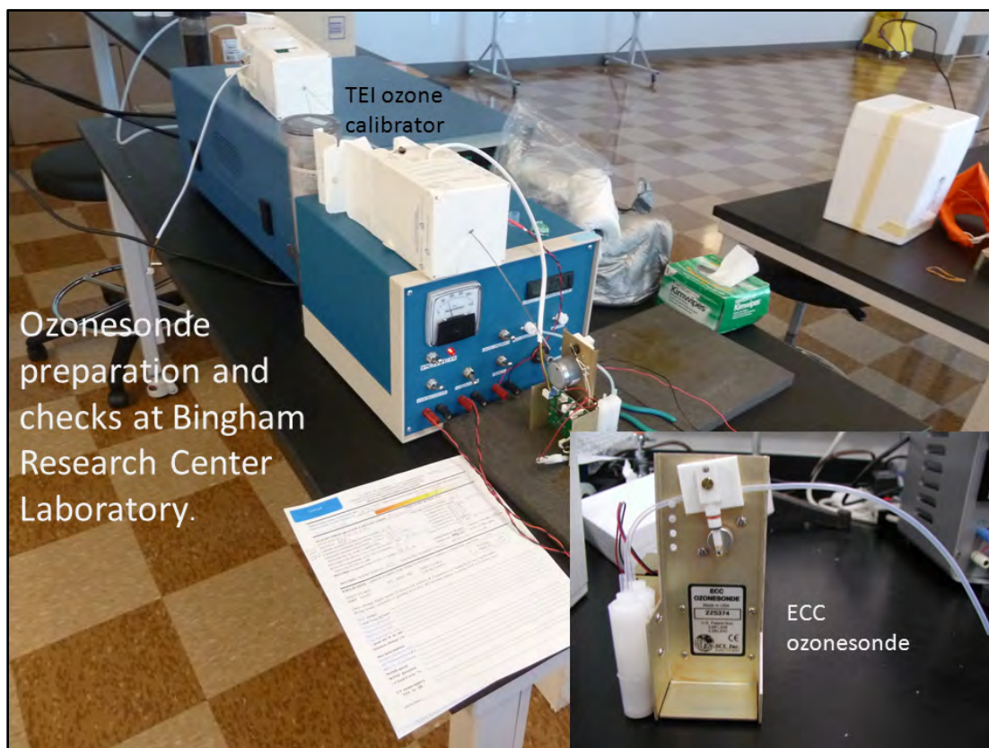
Figure 5B-3. Ozonesonde preparation and testing location in Bingham Research Center Laboratory. Every ozonesonde used in the Uintah Basin program was tested and calibrated before use.
