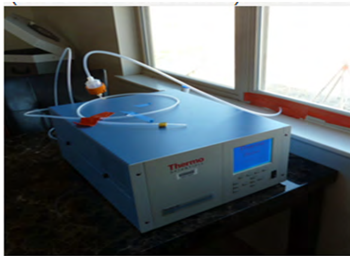
Figure 5B-2. UV photometric surface ozone analyzer TEI operated full time at the Ouray site during the February campaign.
