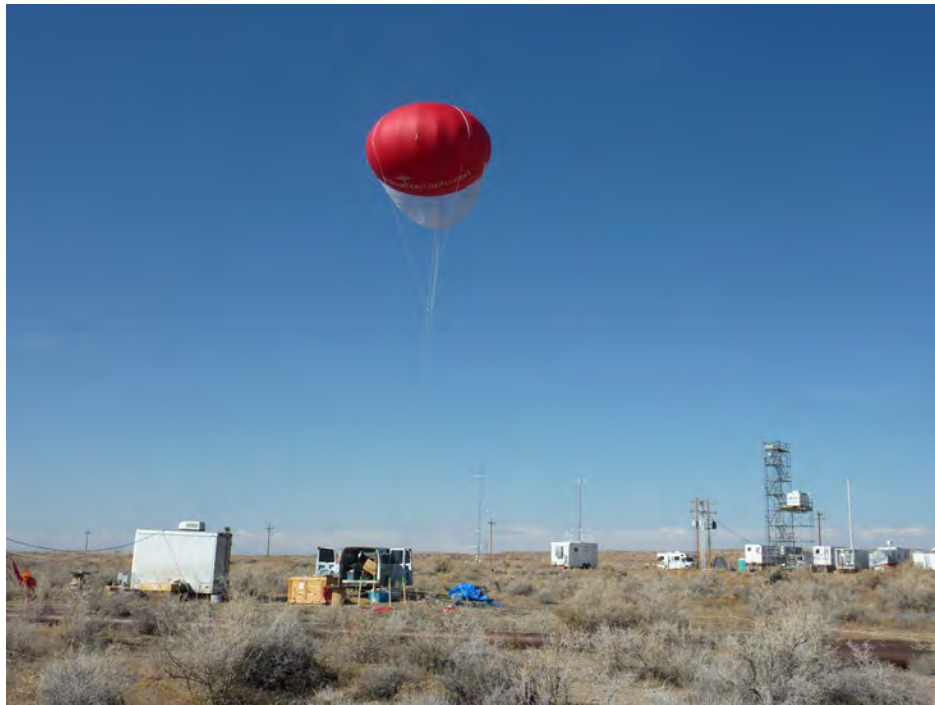
Figure 6-1. Setup of the CU Boulder experiment at the Horsepool site. The photograph depicts the 20-foot diameter SkyDoc tethered balloon, the balloon winch (inside wooden box), and the CU instrument trailer. At the time of the picture, the balloon was lowered to the surface (here at approximately 30 feet) for instrument maintenance. During regular operation, the balloon was raised to 500 feet and served as a “sky dock” for raising instruments and sampling-line inlets.
