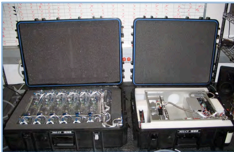
Figure 5A-4. NOAA discrete air sampling system close-up. On the left is the Programmable Flask Package (also called 12-pack or PFP), which contains 12 glass flasks (0.7L each). On the right is the Programmable Compressor Package (PCP), which contains pumps for flushing the manifold and flask prior to pressurizing the flask to approximately 40 psia.
