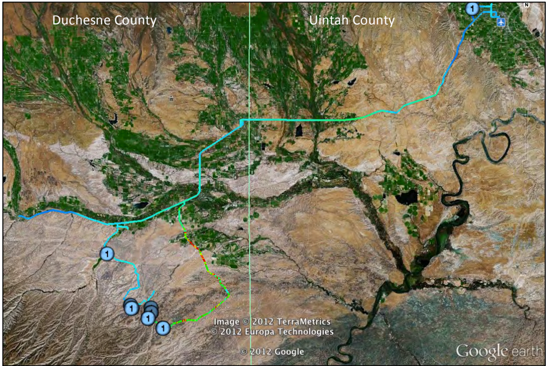
Figure 5A-14. Map of February 11, 2012 survey track, color coded with methane mixing ratio (from 1.8 ppm in blue to 3.8ppm and beyond in red). Blue balloons show the discrete flasks sampling locations.
