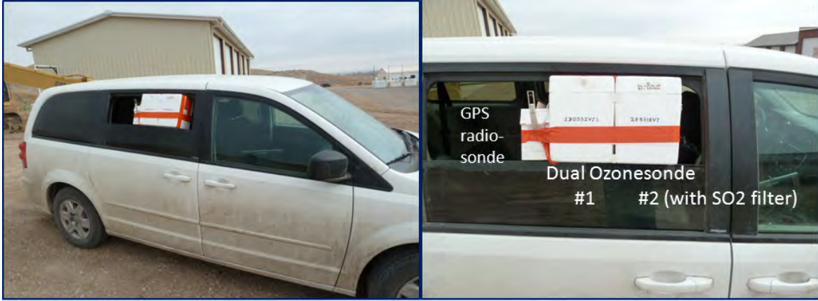
Figure 5B-11. NOAA dual ozonesonde instrument mounted for mobile measurements.
